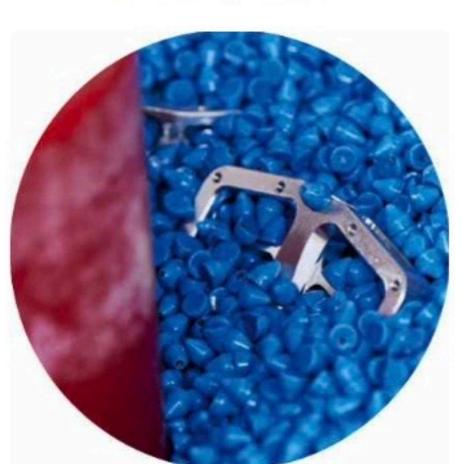
3. After machining, the parts are put in a rumbler to smooth the rough edges, then anodised, laser-etched with the PEMBREE logo, assembled and packaged up ready to be shipped out to customers.
