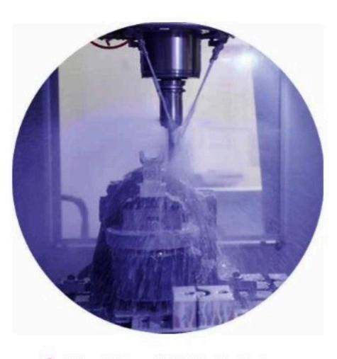
2. Aluminium billet is fed into a fully-automated seven-axis Haas CNC machine. This uses the data from Autodesk 360 to carve the metal into raw components.
